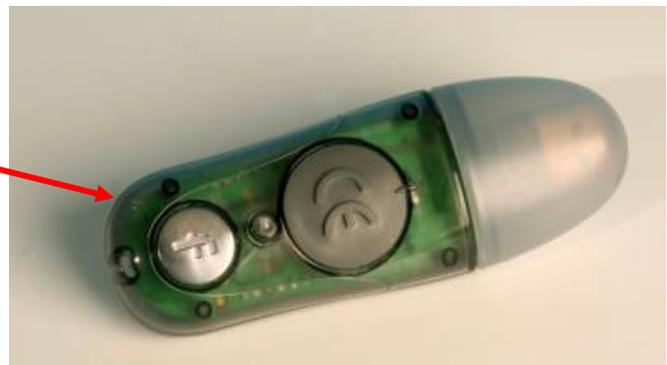
Figure 1: Termologger USB battery compartment
