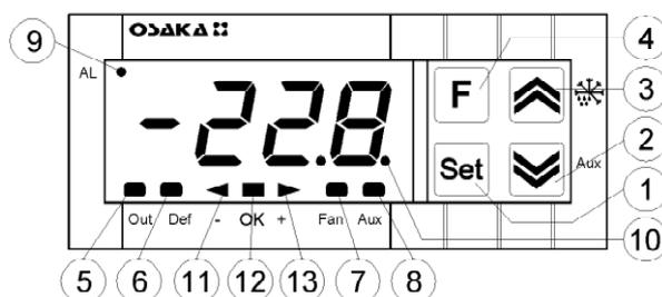
**1 - Key Set** : Used for setting the Set point and for programming the function parameters
