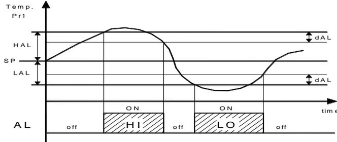
The maximum and minimum temperature alarms can be disabled by setting the relative parameters "HAL" and "LAL" = OFF.
