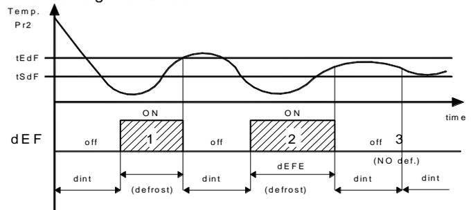
**Examples:** defrosting 1 ends due to reaching of temperature "tEdF", defrosting 2 ends at the end of the "dEFE" time as the temperature "tEdF" is not reached, defrosting 3 does not take place as the temperature is higher than "tSdF".
