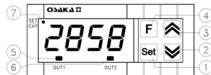
1 - **Key Set**: Used for the set point setting and to program the functioning parameters
