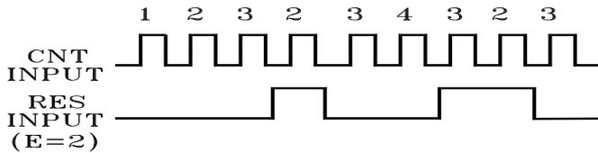
In this operation mode it is necessary to pay attention at counting speed because the Reset input have a delay of 15 m sec. and therefore the inversion of the calculation is not instant.
