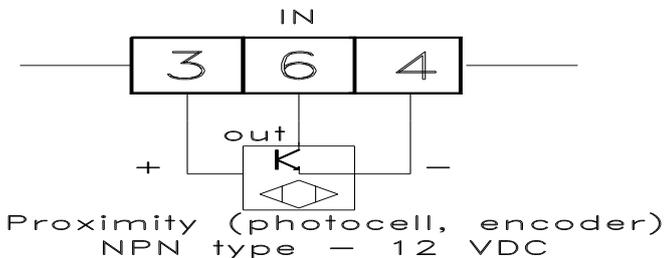
In order to the counting frequency is advisable to program the filter software of the par. "H" that it allows to select the maximum counting frequency and to avoid false counting (for instance caused by the contacts rebounds).
